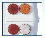
LED clearance lights, direction lights, stop lights and back-up lights are standard equipment offering enhanced safety, while reducing operating and maintenance costs.
